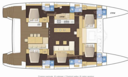
Cuisine centrale, 6 cabins / Central galley, 6 cabin version
