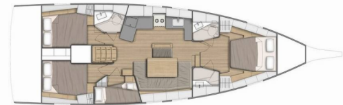
OCEANIS 46.1 - layout 4 CABINS & 2 HEADS
